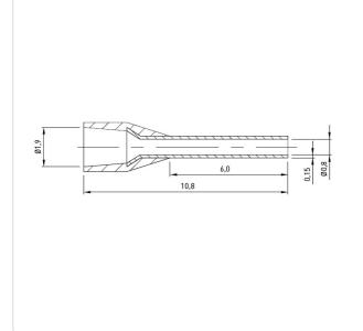
Color: Yellow Finish: **Tin-Plated** Insulation: Polypropylene Length [mm]: 11 **Electrolytic Copper** Material: Material Group: **Electrolytic Copper** Plug-In Length [mm]: 6 Wire Cross Section [mm<sup>2</sup>]: 0.25 Weight: 0.04g Conformities:
