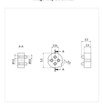
Length [mm]: 3.5 Material: PA 6.0 Material Group: **Plastic** Model: TO-18 Outer Diameter [mm]: 5.5 Weight: 0.08g
