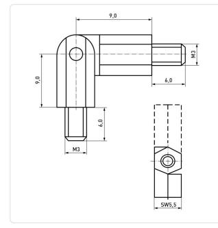
Finish: Nickel-Plated, 3 µm, E1E Leg Length 1 [mm]: 9 Leg Length 2 [mm]: 9 Length [mm]: 18 Material: Brass Material Group: Brass Model: Male/Male M3 Thread 1 Size: Thread 2 Size: М3 Weight: 4.18g Conformities: SVHC Reach RoHS
