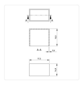
Color: Black Flammability Class: UL94-V2 Height [mm]: 10.5 17.3 Length [mm]: PA 6.6 Material: Material Group: **Plastic**
