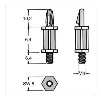
Color: Natural Flammability Class: UL94-V2 6.4 Length [mm]: Material: PA 6.6 Material Group: **Plastic** PCB Hole Ø [mm]: PCB Thickness [mm]: 1,6 Thread Size: M4
