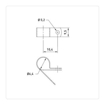
Bundle Diameter [mm]: 6,4 Color: Natural Distance Middle/Middle [mm]: 10.4 UL94-V2 Flammability Class: Material: PA 6.6 Material Group: Plastic Mounting Hole [mm]: 5.2 Thickness [mm]: 1.3 Width [mm]: 9.5 Weight: 0.55g
