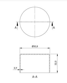
Color:BlackFlammability Class:UL94-V0Height [mm]:32Material:DAP - DiaMaterial Group:PlasticModel:EnclosuraWidth [mm]:50.8Weight:12gConformities:Reach
