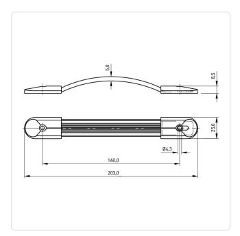
Color: Black Dist. Mounting Holes [mm]: 160 Height [mm]: 8.5 Material: Plastic Material Group: Plastic
