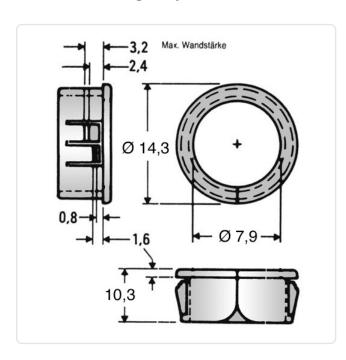
Color: Black Inner Diameter [mm]: 8 Material: PA 6.6 Material Group: Plastic Max. Panel Thickness [mm]: 3.2 Mounting Hole [mm]: 12.7
