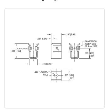
Amperage [A]: 15 Fuse Size [mm]: 5.0x20.0 Material: **Brass** Material Group: **Brass** Model: Clip Holder
