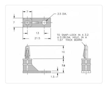
Color: Natural Flammability Class: UL94-V2 Length [mm]: 7.6 Material: PA 6.6 Material Group: **Plastic** Panel Hole Ø [mm]: 3.5
