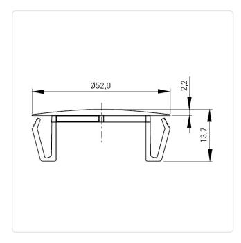
Color: Black Head Diameter [mm]: 52 Head Height [mm]: 2.2 PA 6.6 Material: Material Group: **Plastic**
