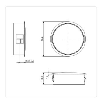
Color: White Flammability Class: UL94-V2 Head Diameter [mm]: 19.8 Head Height [mm]: 1.6 PA 6.6 Material: Material Group: Plastic Snap-In Model: Mounting Hole [mm]: 17.5
