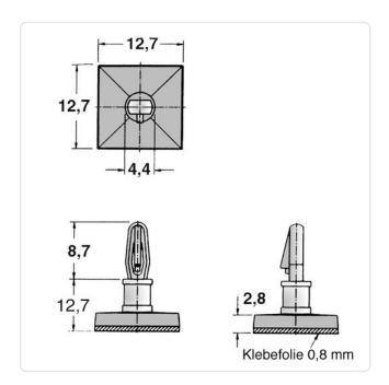
Color: Natural Flammability Class: UL94-V2 Length [mm]: 12.7 Material: PA 6.6 Material Group: **Plastic** PCB Hole Ø [mm]: 3.2 PCB Thickness [mm]: 1,6 Weight: 0.62g
