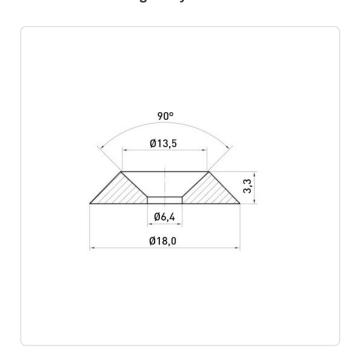
Finish: Plain For Thread Size: M6 Height [mm]: 3.3 Inner Diameter [mm]: 6.4
