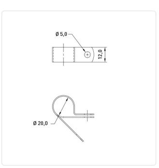
Bundle Diameter [mm]: 20 Color: Black Material: PA 6.6 Plastic Material Group: Mounting Hole [mm]: 5 Width [mm]: 12 Weight: 1.53g
