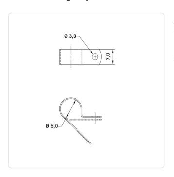
Bundle Diameter [mm]: 5 Color: Black Material: PA 6.6 Plastic Material Group: Mounting Hole [mm]: 3
