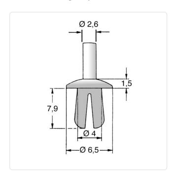
Color: Black UL94-V2 Flammability Class: Head Diameter [mm]: 6.5 Head Height [mm]: 1.5 Length [mm]: 7.9 Mandrel Diameter [mm]: 2.6 PA 6.6 Material: Material Group: Plastic
