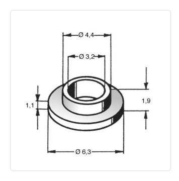
Color: Black Flammability Class: UL94-V0 1.9 Height [mm]: Inner Diameter [mm]: 3.2 Lug Diameter [mm]: 4.4
