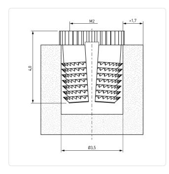
Finish: Plain Length [mm]: 4 Material: **Brass** Material Group: Brass Minimum Edge Distance [mm]: 1.7 Panel Hole Ø [mm]: 3.5 Thread Size: M2
