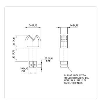
Bundle Diameter [mm]: 5,0-10,0 Color: Natural Height [mm]: 7.7 PA 6.6 Material: Material Group: **Plastic** Mounting Hole [mm]: 3.8 Panel Thickness [mm]: 2,0mm Width [mm]: 9.1 Weight: 0.2g
