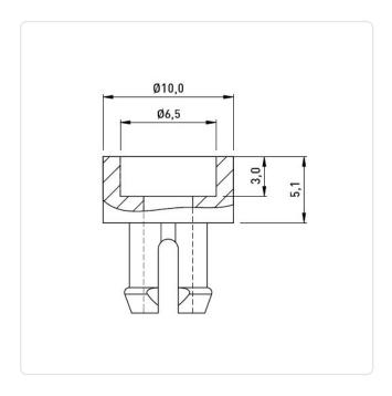
Color: Natural Flammability Class: UL94-V2 For Thread Size: M3.5 Inner Diameter [mm]: 6.5 Length [mm]: 5.1 Material: PA 6.6 Material Group: Plastic Mounting Hole [mm]: 6.5 Outer Diameter [mm]: 10 Weight: 0.4g
