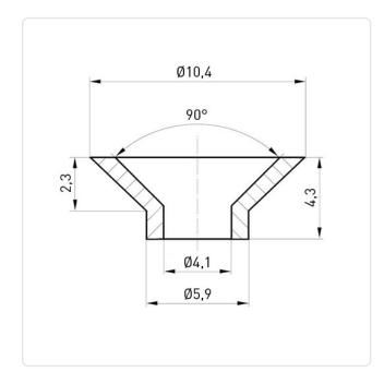
Color: Natural Flammability Class: UL94-V2 Inner Diameter [mm]: 4.1 Lug Diameter [mm]: 5.9 Material: PA 6.0
