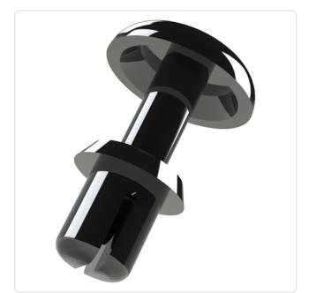
Color: Black UL94-V2 Flammability Class: Head Diameter [mm]: 4.2 Head Height [mm]: 1.2 Length [mm]: 3.2 Material: PA 6.0 Material Group: Plastic Model: removable Mounting Hole Range [mm]: Ø 2.1-2.2
