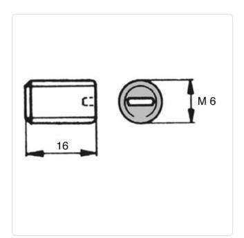
Color: Natural DIN/ISO: ISO4766 Drive Type: Slotted Flammability Class: UL94-V2 Length [mm]: 16 Material: PA 6.6 Material Group: Plastic Point Type: Flat Point Thread Size: M6
