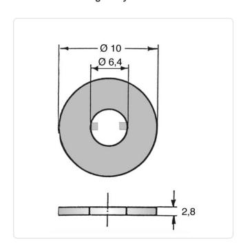
Color: Natural For Thread Size: M6 Height [mm]: 2.8 Inner Diameter [mm]: 6.4 Material: PA 6.0 Material Group: Plastic Outer Diameter [mm]: 10 Weight: 0.14g
