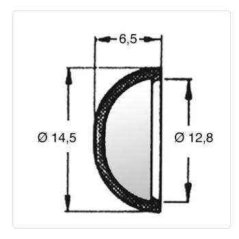
Color: Gray Head Height [mm]: 6.5 Inner Diameter [mm]: 12.8 PA 6.0 Material: Material Group: **Plastic**
