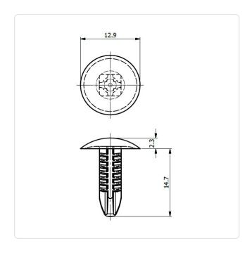
Color: Black Flammability Class: UL94-V2 Head Diameter [mm]: 12.9 Head Height [mm]: 2.3 Length [mm]: 14.7 Material: PA 6.6 Material Group: **Plastic** Mounting Hole [mm]: Panel Thickness [mm]: 1,5-7,5 Weight: 0.22g
