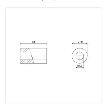
Color: Russet Flammability Class: UL94-V0 For Thread Size: M4 Inner Diameter [mm]: 4.5
