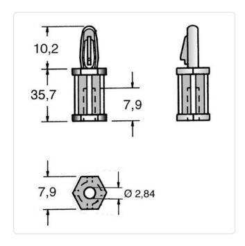
Color: Natural Flammability Class: UL94-V0 35.7 Length [mm]: Material: PA 6.6 Material Group: **Plastic** PCB Hole Ø [mm]: PCB Thickness [mm]: 1,6 Thread Size: M3.5
