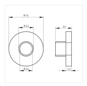
Color: Natural Flammability Class: UL94-V0 2.4 Height [mm]: Inner Diameter [mm]: 3.6 Lug Diameter [mm]: 4.32 Material: PA 6.6
