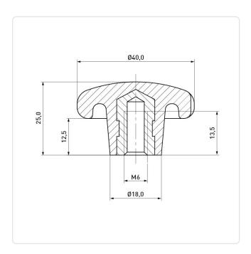
Color: Black Diameter [mm]: 40 Height [mm]: Material: Plastic Material Group: Plastic Thread Size: M6 Weight: 19.2g Conformities:
