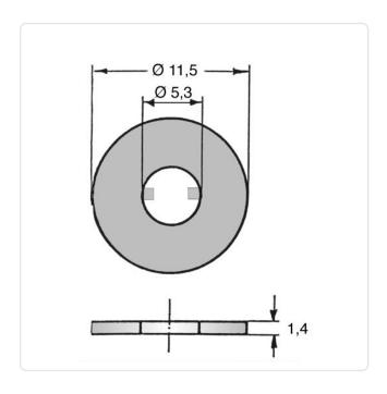
Color: Natural For Thread Size: M5 Height [mm]: 1.4 Inner Diameter [mm]: 5.3 Material: PA 6.0 Material Group: Plastic Outer Diameter [mm]: 11.5 Weight: 0.11g
