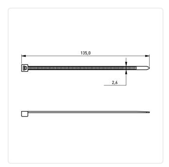
Bundle Diameter [mm]: 25,0-30,0 Color: Natural Flammability Class: UL94-V2 135 Length [mm]: Material: PA 6.6 **Plastic** Material Group: 2.5 Width [mm]:
