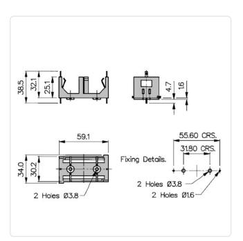
Battery Type: C-Baby Flammability Class: UL94-HB
