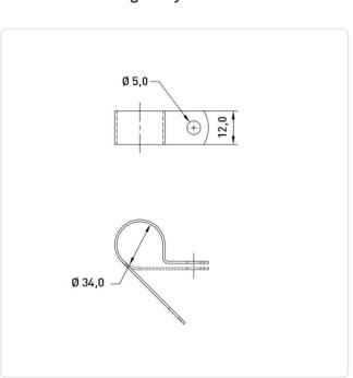
Bundle Diameter [mm]: 34 Color: Black Material: PA 6.6 Plastic Material Group: Mounting Hole [mm]: 5 Width [mm]: 12 Weight: 1.46g
