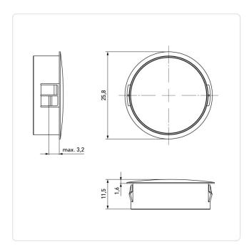
Color: White Flammability Class: UL94-V2 Head Diameter [mm]: 25.8 Head Height [mm]: 1.6 PA 6.6 Material: Material Group: Plastic Snap-In Model: Mounting Hole [mm]: 22.2
