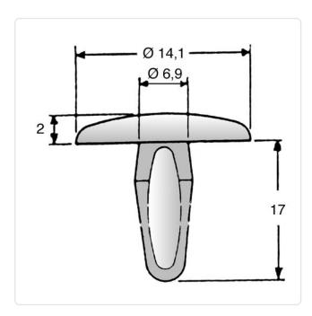
Color: Black Flammability Class: UL94-V2 Head Diameter [mm]: 14.1 Material: PA 6.0 Material Group: **Plastic**
