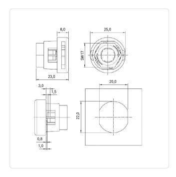
Cable diameter [mm]: Ø 8,5-9,5 Color: Natural Diameter [mm]: 25 PA 6.0 Material: Material Group: Plastic Max. Panel Thickness [mm]: 3
