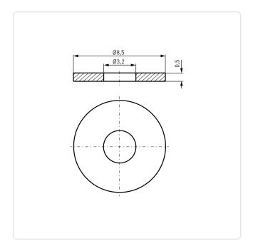
Color: Black For Thread Size: М3 Height [mm]: 0.5 Inner Diameter [mm]: 3.2
