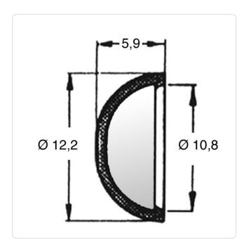
Color: White Head Height [mm]: 5.9 Inner Diameter [mm]: 10.8 Material: PA 6.0 Material Group: **Plastic**
