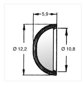
Color: Black Head Height [mm]: 5.9 Inner Diameter [mm]: 10.8 PA 6.0 Material: Material Group: **Plastic**
