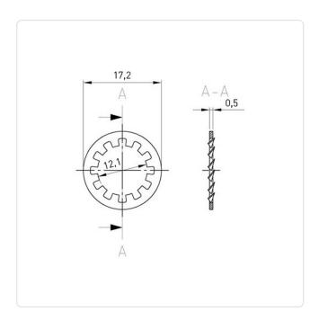
Finish: Alkaline Galvanized 8 µm
