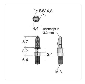
Color: Natural Flammability Class: UL94-V2 3.2 Length [mm]: PA 6.6 Material: Material Group: **Plastic** PCB Hole Ø [mm]: 3.2 PCB Thickness [mm]: 1,6 Thread Size: М3
