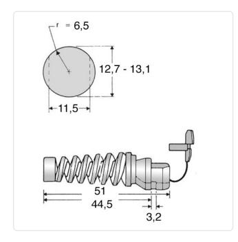
Cable diameter [mm]: Ø 3,0-7,6 Color: Black Material: PA 6.6 Material Group: Plastic Max. Panel Thickness [mm]: 3.2 Mounting Hole [mm]: 12.7 Panel Thickness Range [mm]: 6,4-7,4
