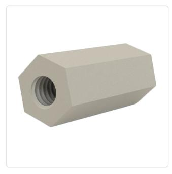
Color: Natural Flammability Class: UL94-V2 Length [mm]: 15.9 Material: PA 6.6 Material Group: **Plastic** Profile: Hexagonal Thread 1 Length [mm]: 15.9 Thread 1 Size: UNC4-40 Weight: 0.63g
