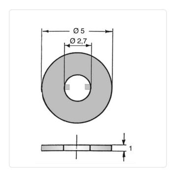
Color: Natural For Thread Size: M2.5 Height [mm]: Inner Diameter [mm]: 2.7 Material: PA 6.0 Material Group: Plastic Outer Diameter [mm]: 5
