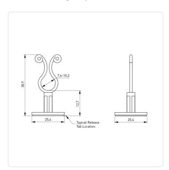
Bundle Diameter [mm]: 3,0-10,0 Color: Natural Flammability Class: UL94-V2 Material: PA 6.6 Material Group: **Plastic**
