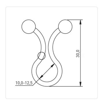
Bundle Diameter [mm]: 10,0-15,0 Color: Natural Flammability Class: UL94-V2 Material: PA 6.6 Material Group: Plastic Weight: 0.39g
