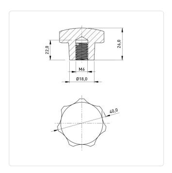
Color: Black Diameter [mm]: 40 Height [mm]: Material: PA 6.0 Material Group: Plastic Thread Size: M6 Weight: 14.2g
